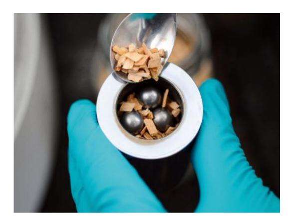
The first step in reaching the treasure in lignin: Wood chips are ground down in a ball mill and mixed with sulphuric acid. The acid splits the biopolymer into its individual components. Thanks to a new approach discovered by the Mülheimbased chemists, these can also be processed more effectively. Credit: Frank Vinken
