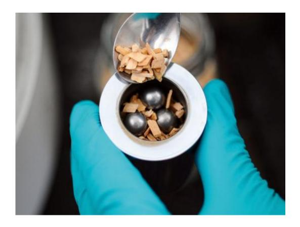
The first step in reaching the treasure in lignin: Wood chips are ground down in a ball mill and mixed with sulphuric acid. The acid splits the biopolymer into its individual components. Thanks to a new approach discovered by the Mülheimbased chemists, these can also be processed more effectively. Credit: Frank Vinken
