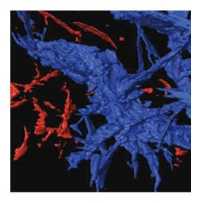
In a rock and metal sample created by Stanford scientists to mimic the make up of the early Earth mantle, drops of molten iron merge to form a network. In this X-ray tomography image of the sample, the channels labeled in blue are interconnected. Credit: Crystal Shi
