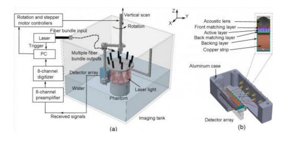
This is a schematic illustration of the imaging system and the ultrasound detector. Credit: Wenfeng Xia, Biomedical Photonic Imaging group, University of Twente
