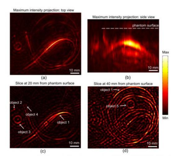
The top image shows a top and side view of a 3-D-reconstructed phantom object made of gels and other materials that mimic human tissue. The background of this phantom mimics normal breast tissue, while several objects embedded within the material mimic blood vessels and tumors. The bottom image shows
