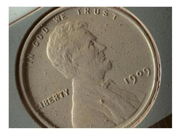
This image of a U.S. penny was acquired Mars Hand Lens Imager (MAHLI) aboard NASA's Curiosity rover in northern Gale crater on Mars. At 14 micrometers per pixel, this is the highest resolution image that the MAHLI can acquire. The image shows that, during the penny's 14 months (so far) on Mars, it has accumulated Martian dust and clumps of dust, despite its vertical mounting position. Credit: NASA/JPL-Caltech/MSSS/Planetary Science Institute
