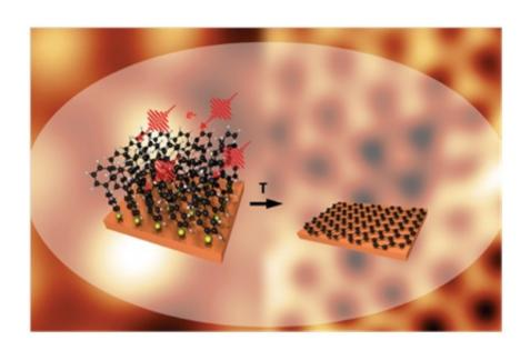
The cover picture of the scientific journal "*Advanced Materials*" gives a schematic representation of the conversion of the monolayer of the complex molecule biphenyl thiol in the two-dimensional graphene crystal by electron irradiation and thermal treatment. Credit: Copyright Wiley-VCH Verlag GmbH & Co. KGaA. Reproduced with permission.
