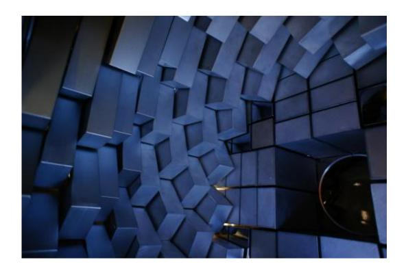
The DALI2 gamma-ray detector array at the Radioactive Isotope Beam Factory, Japan, which was used to deduce the energies of the nuclear excited levels reported in the present study. Credit: Dr Satoshi Takeuchi
