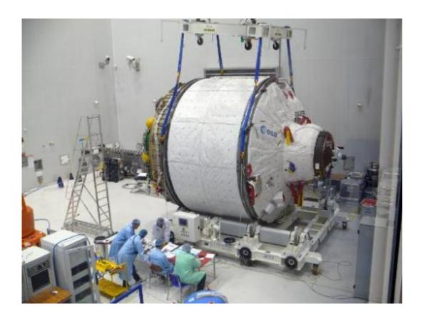
The ICC portion of the Automated Transfer Vehicle Albert Einstein, the fourth in a series of lifeline vessels bringing supplies and critical altitude boosts to the International Space Station, being weighed at Kourou space center, French Guiana
