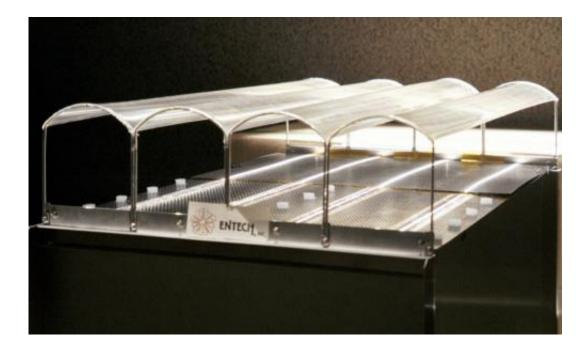
In the Stretched Lens Array, a descendant of SCARLET, a thin film studded with tiny prisms is stretched between arches to help it focus sunlight onto solar cells below.
