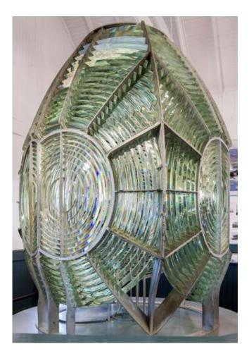
The Fresnel lenses that serve lighthouses consist of concentric rings, each of which refracts light as the corresponding part of a regular lens would do.
