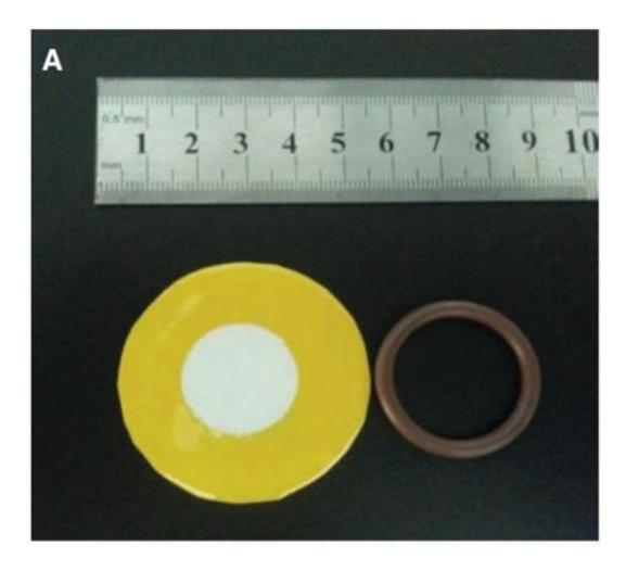
Digital picture of an ultrathin GO membrane on AAO (~9 nm). The white circular area is the permeation area (~4 cm2) with supported GO; the yellow Kapton tape is used for GO protection and sealing by an O-ring during permeation measurements. Credit: *Science*, 2013. DOI: 10.1126/science.1236686
