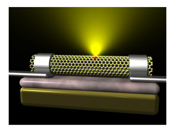
This is a diagram of the device proposed by the UPV/EHU's NanoBio Spectroscopy Group. The result has led to the patent for a new source of light emission; its main feature is that it emits across the whole of the visible and ultraviolet spectrum at ambient temperature, and can be produced using standard manufacturing methods. Credit: UPV/EHU
