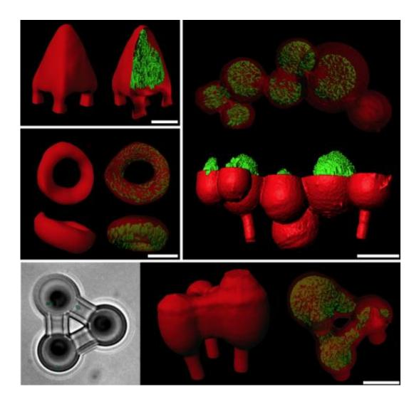
The researchers use a novel 3-D printing technology to build homes for bacteria at a microscopic level. The resulting structures (imaged in red through confocal fluorescence) can be of almost any shape or size, and can be moved around in relationship to other structures containing bacterial microcommunities (imaged in green). Credit: Jason Shear
