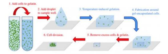
The bacteria are put in the solution, and when the solution cools, the bacteria become fixed in place. The researchers then identify which bacteria they want to cage and in what shape and fire the laser, using a chip adapted from a digital movie projector to project a two-dimensional image into the gelatin. Wherever it focuses, a solid matrix forms. Credit: Jason Shear
