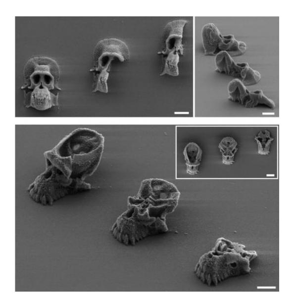
This three-dimensional chimpanzee skull was printed using the same basic technology that Shear's lab is now using to print bacterial cages. Credit: Jason Shear
