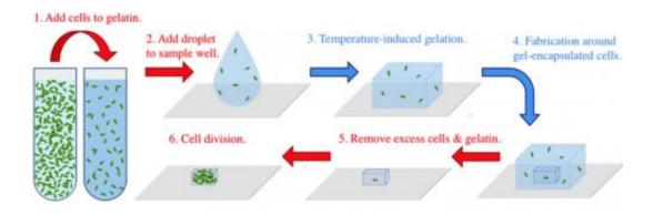
The bacteria are put in the solution, and when the solution cools, the bacteria become fixed in place. The researchers then identify which bacteria they want to cage and in what shape and fire the laser, using a chip adapted from a digital movie projector to project a two-dimensional image into the gelatin. Wherever it focuses, a solid matrix forms. Credit: Jason Shear
