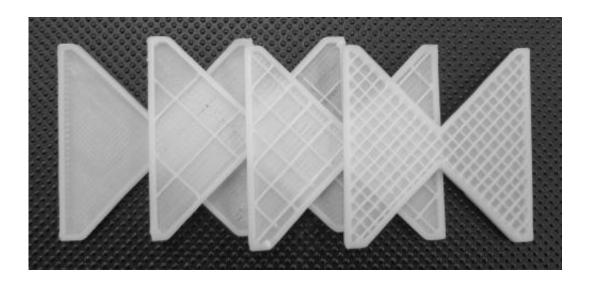
One way 3-D printing saves energy over manufacturing is by using less raw material. This series of partially printed Swiss children's blocks illustrates how a 3-D printer can partially fill the interior of an item with plastic while maintaining its structural strength. Credit: Samuel Bernier/Thingiverse.com
