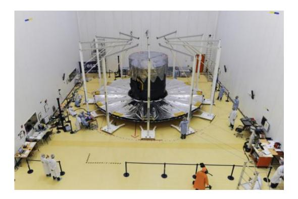
The Gaia Deployable Sunshield Assembly (DSA) during deployment testing in the S1B integration building at Europe's spaceport in Kourou, French Guiana, on 10 October 2013. Credit: ESA–M. Pedoussaut, 2013
