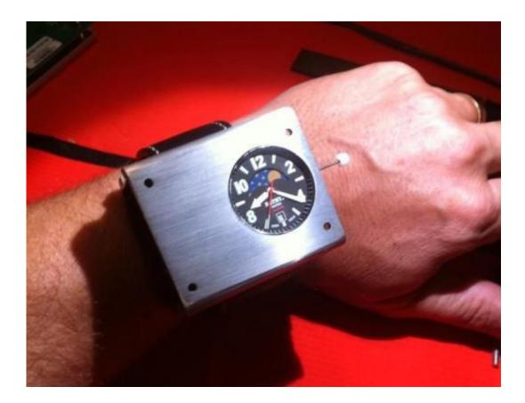
Bathys Hawaii, a US-based watch company, has created the Cesium 133, a prototype wrist watch that has its own atomic clock. The fact that the clock is self-contained, integrated into the wristwatch, is the distinguishing factor. The clock does not need to collect information
