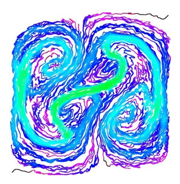
This is an instantaneous illustration of the lamination observed during a cat's eyes flip mixing sequence. Credit: L.Rossi/CEA
