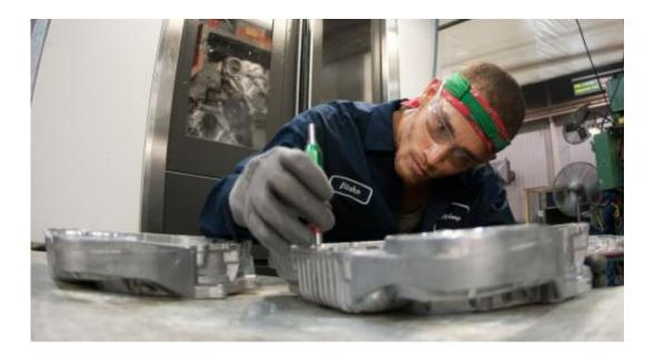
Machine operator Blake Veeneman inspects a high-pressure aluminum casting in a factory at Muskegon, Mich., that makes automotive components. Credit: Lance Cheung, U.S. Department of Agriculture
