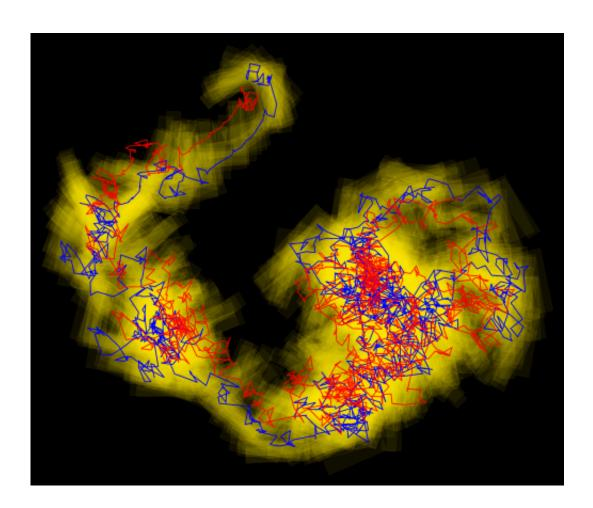
A trajectory of a boomerang particle in water, starting from the top of the image, with the blue line tracking the point where the arms meet and the red line tracking the "center of hydrodynamic stress," a point along the axis bisecting the angle of the arms. The boomerang itself is shown in yellow. Credit: A. Chakrabarty et al., Phys. Rev. Lett. (2013)
