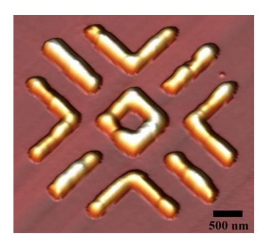
This pattern represents the logo of Moncloa Campus, a topographic image taken with an atomic force microscope of biomimetic polymeric material developed by electron beam lithography. Credit: UPM
