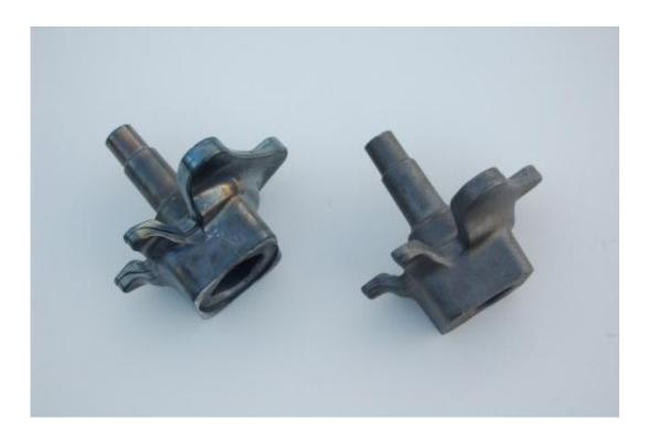
Following years of research, the technology involving thixoforming, in other words, the shaping of metals in a semi-solid state, is beginning to yield results. CIC marGUNE, the Co-operative Research Centre for High-performance Manufacturing, is exploring the possibility of modifying the current process to manufacture parts for the automotive industry, thanks to thixoforming technology. This research is being
