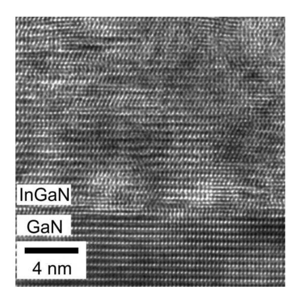
The atomic arrangement at a relaxed InGaN/GaN interface created by layer-by-layer atomic crystal growth is shown. The technique may point to new developments in solar cell efficiency. Credit: Arizona State University
