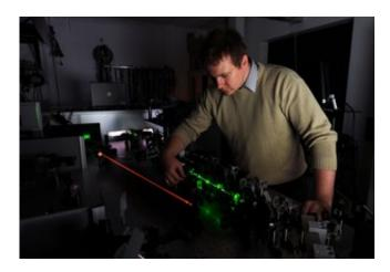
New parametric amplifier developed in the Laser Centre at the Institute of Physical Chemistry of the Polish Academy of Sciences in Warsaw and the Faculty of Physics of the Warsaw University allows for constructing desktop-size laser setups capable of generating femtosecond laser pulses with a power of tens of terawatts. Pictured above: Dr Paweł Wnuk from the Laser Centre at the new amplifier. Credit: IPC PAS, Grzegorz Krzyżewski
