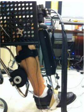
A front and side view of a volunteer wearing the Anklebot in a seated posture. During experiments, the robot moved the ankle and recorded its stiffness in multiple directions. Credit: HYUNGLAE LEE
