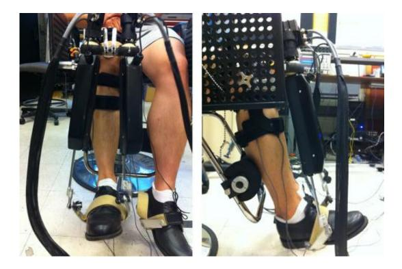
A front and side view of a volunteer wearing the Anklebot in a seated posture. During experiments, the robot moved the ankle and recorded its stiffness in multiple directions. Credit: HYUNGLAE LEE
