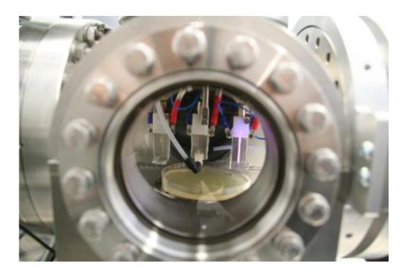
Plasma reactor: The RUB team generates atmospheric-pressure plasmas and tests which effects UV radiation and reactive particles have on bacterial cells and molecules. Credit: © RUB, Foto: Jan-Wilm Lackmann
