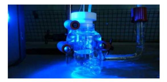
Electrodes in a test cell to produce hydrogen with light. Credit: Erwin Reisner
