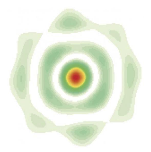
This is the reconstruction of the two-dimensional focus field. The intensity is color coded. Credit: University of Göttingen
