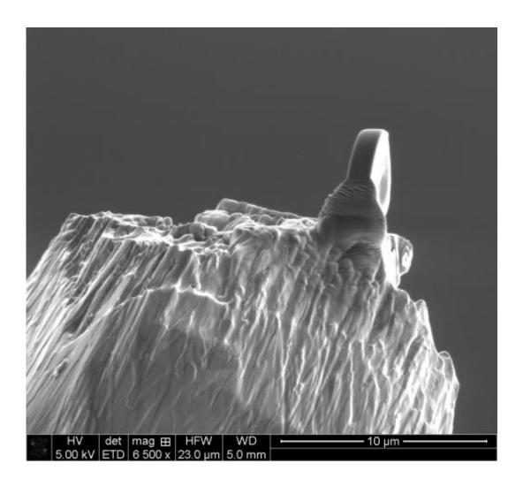
This is an electron micrograph of the micro lens on the tip of a needle. The lens has a diameter of just two microns (thousandths of a millimeter). Credit: University of Göttingen
