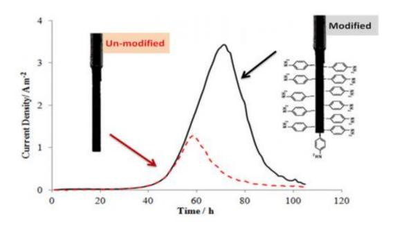
This shows wiring microbes to conduct and produce electricity faster. Credit: Amit Kumara
