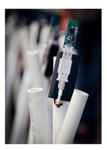
This is a wireless sensor, similar to those used in home wireless networks, used to detect falls using radio waves. University of Utah researchers used an array of sensors around a room to determine whether someone inside the network was standing or falling. Credit: Dan Hixson, University of Utah.
