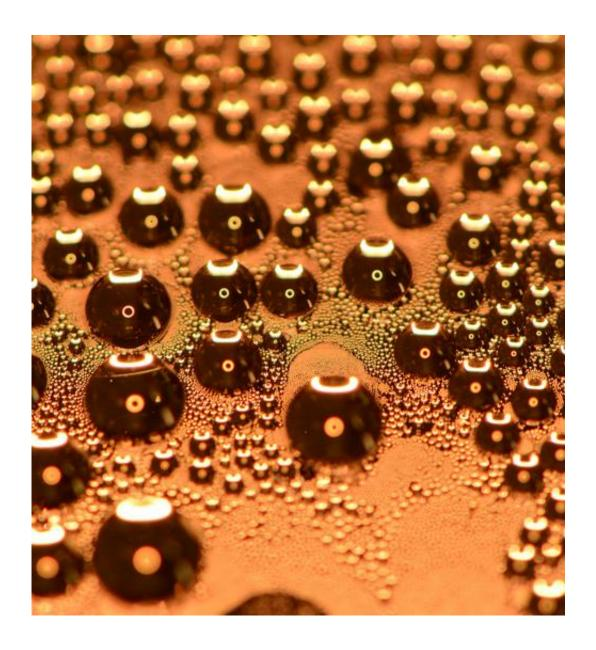
On typical hydrophobic coatings, seen here, droplets forming from high-temperature steam soon spread out to coat the surface (as is beginning to happen at the bottom), quickly degrading their performance. The new coating maintains its ability to foster droplet formation over long periods. Credit: RESEARCHERS
