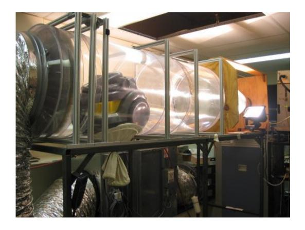
A vacuum is tested inside the clean air wind tunnel. Credit: Caroline Duchaine
