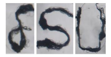
Eden Steven tested whether his spider silk wires would conduct electricity when bent — they did.
