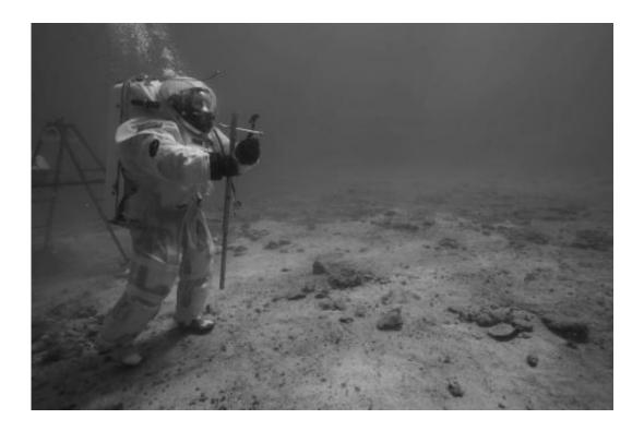
ESA astronaut instructor Hervé Stevenin ready to perform soil core sampling with a core tube and a hammer underwater off the coast of Marseille. During the mission, several soil samples were collected by the aquanauts with similar tools used on the Moon by the Apollo 11 crew. Credit: Alexis Rosenfeld
