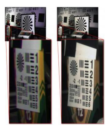
These insets show the resolution of a conventional wide-angle lens (left) compared to that of the new fiber-coupled monocentric lens system (right), where both images were captured with identical 5Mpixel focal planes. Credit: UCSD Jacobs School of Engineering
