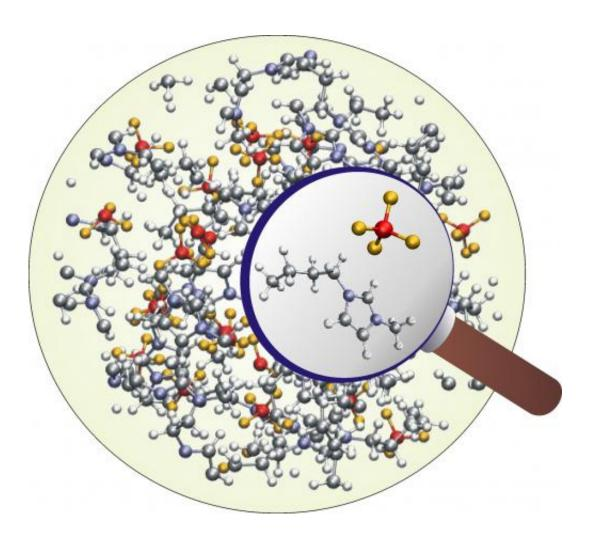
Computer simulation of an ionic solvent The image shows a computer simulation of a frequently-used ionic solvent. NOE experiments at low frequencies capture the structure of the entire area. Experiments at high frequencies provide information regarding the local structure of two neighbouring particles, highlighted by the magnifying glass.
