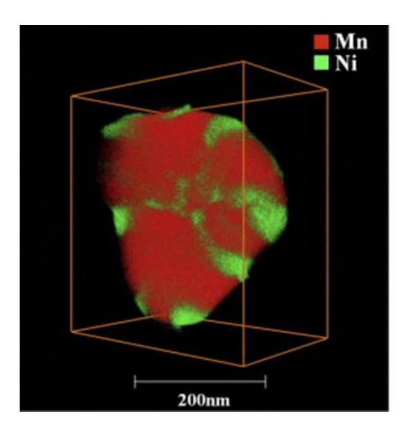
A new technique combining scanning transmission electron microscopy and X-ray energy dispersive spectrometry showed this 3D nanoparticle used as a cathode material in lithium ion batteries. The technique enables clearer
