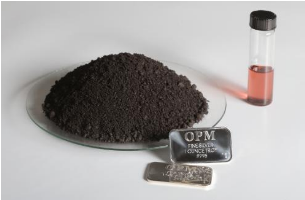
Dish containing 140 grams of silver nanoparticle powder pictured with a solution of the nanoparticles and 2 troy ounces of silver bullion, which is approximately the quantity of silver contained in the pile. Credit: Daniel Miller
