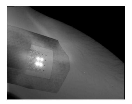
In this infrared image, active heating elements of an ultrathin device on the skin appear white due their increased temperature. The device construction allows for application of controlled heating while simulataneously mapping temperature changes to 0.02 °C. Credit: University of Illinois and Beckman Institute
