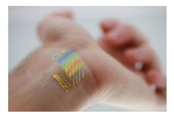
An ultrathin device for mapping changes in skin temperature to  $0.02 \,^{\circ}$ C is shown with a representative colormap of temperature distribution on the wrist. Credit: University of Illinois and Beckman Institute
