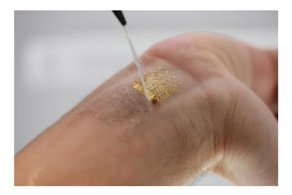
An ultrathin device for mapping changes in skin temperature to 0.02 °C is applied to the skin using a water-soluble backing. Credit: University of Illinois and Beckman Institute
