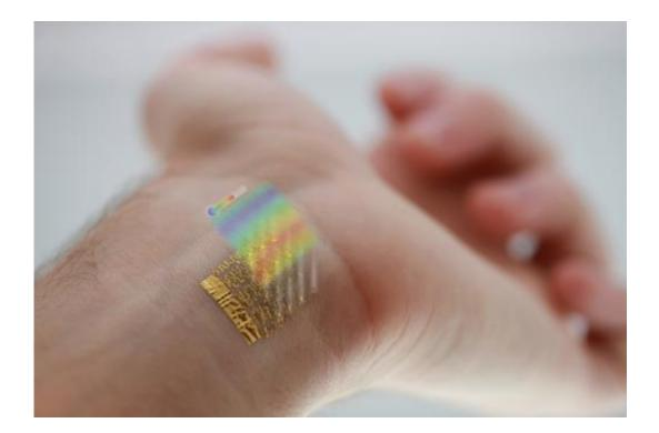
An ultrathin device for mapping changes in skin temperature to  $0.02\,^{\circ}\text{C}$  is shown with a representative colormap of temperature distribution on the wrist. Credit: University of Illinois and Beckman Institute
