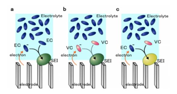
Figure 3 in the press release document: (a) The reaction mechanism of the formation of an SEI film in the EC solvent without using any additive. (b) The conventional scenario of VC additive effect where VC is sacrificially reduced and decomposed. (c) The VC additive effect on the initial SEI formation elucidated in this research, where VC terminates EC anion radical. This mechanism shows consistency with several experimental observations.
