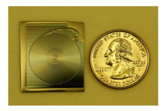
A photograph of the spiral chip-based optical resonator developed at caltech, shown next to a quarter to provide scale. Credit: Hansuek Lee/Caltech
