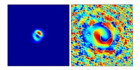
These images shows the spiral structure of the coherent OAM light emitted from a beam of electrons accelerated to nearly the speed of light and arranged into a helix by a simple laser. Left: An intensity map. Note the dark center where the light cancels itself out, resulting in a cross section resembling a doughnut. Right: A phase structure map, clearly showing the helix described by the light. Credit: Hemsing, et al.
