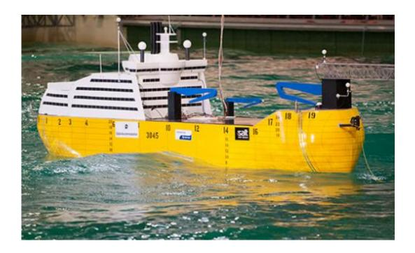
(Phys.org) —A so-called "hotel" ship to accommodate offshore oil rig workers is under construction, which will be engineered in a way to maintain its stability even over rough seas. The new Norwegian ship will make its own waves with internal water tanks. The effort is not only purposed for the comfort of the workers servicing the platforms but for safety. The design will support safe movement from the ship to the platform and precision work while over rough seas. How will this ship
