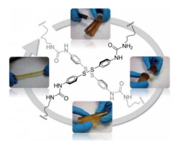
A cylindrical sample of the elastomer mends itself after being cut in two by a razor blade and can be manually stretched without rupture.
