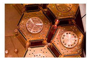
The CDMS experiment uses particle detectors made of germanium and silicon crystals.
