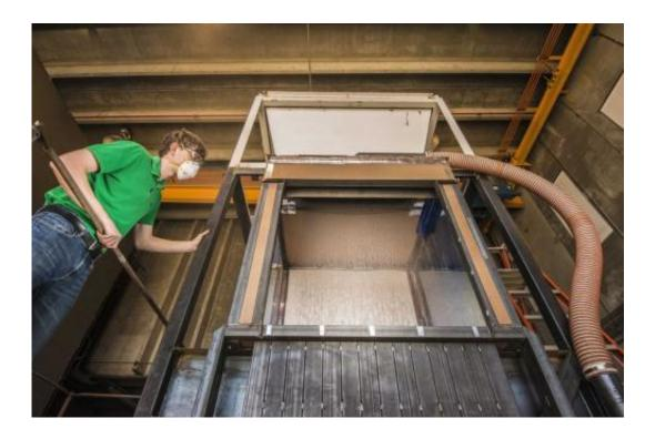
Joshua Mark Christian working with the falling particle receiver, which more efficiently converts the sun's energy to electricity in large-scale, concentrating solar power plants. Credit: Randy Montoya
