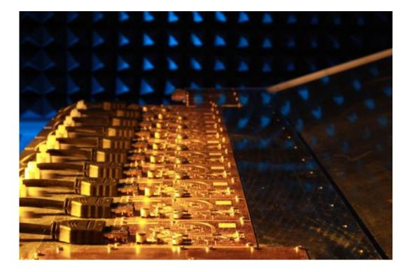
The phased array's transmit/receive modules are equipped with silicongermanium mixed-signal integrated circuits. Credit: Fraunhofer FHR
