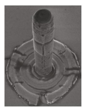
Scanning electron microscope picture of a nanostructure: a semiconductor micropillar with a diameter of 1  $\mu$ m. It consists of a central GaAs layer sandwiched between two so called 'Bragg stacks' made from alternating layers of GaAs and AlAs. The structures are made in Grenoble by molecular-beam-epitaxy and subsequent nanostructuring. Credit: Fundamental Research on Matter (FOM)
