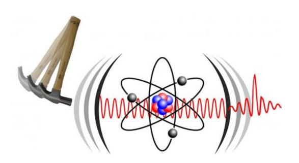
The light source is embedded in an optical resonator where it spontaneously emits a photon. During the emission of the photon the favoured colour of the resonator is quickly switched (symbolised by a hammer) to match the colour of the light source. During this short interval the light source is triggered to emit an burst of photons within a desired moment in time. Credit: Fundamental Research on Matter (FOM)
