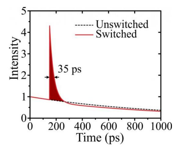
The spontaneous emission intensity from a light source as function of time after excitation at time zero. The usual emission follows an exponential curve (dashed curve). Photons emitted by a light source placed in the switched resonator (red curve) can be bunched within a time window that is much shorter than the average emission time. The short intense burst of light is marked by the red area. Credit: Fundamental Research on Matter (FOM)
