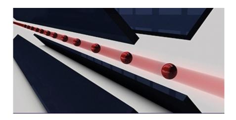
The figure schematically shows a Paul trap with four main electrodes, in which a crystal of Yb+ ions is trapped and overlapped with an optically-trapped cloud of lithium ions. Credit: Ferdinand Schmidt-Kaler
