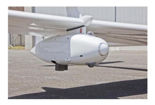
The hyperspectral camera is mounted under the wing of the airplane used for research. Credit: Fraunhofer IFF
