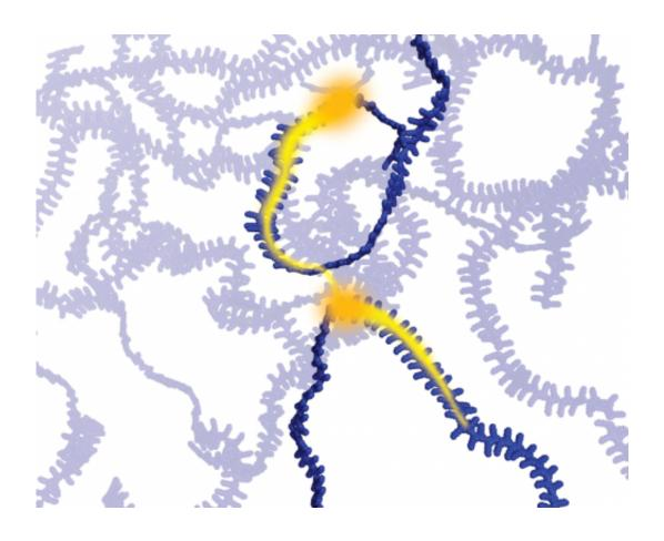
The yellow electric charge races through a "speed-lane" in this stylized view of a polymer semiconductor, but pauses before leaping to the next fast path. Stanford engineers are studying why this occurs with an eye toward building flexible electronics. Credit: Professor Andrew Spakowitz
