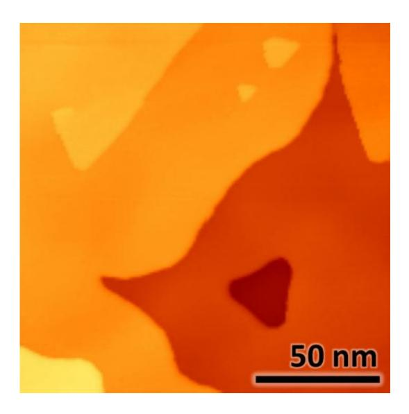
Scanning tunneling microscopy topographic image of a bismuth selenide film grown by molecular-beam epitaxy on a strontium titanate substrate. Terraces with thicknesses between 2 to 5 layers can be found on the same film.
