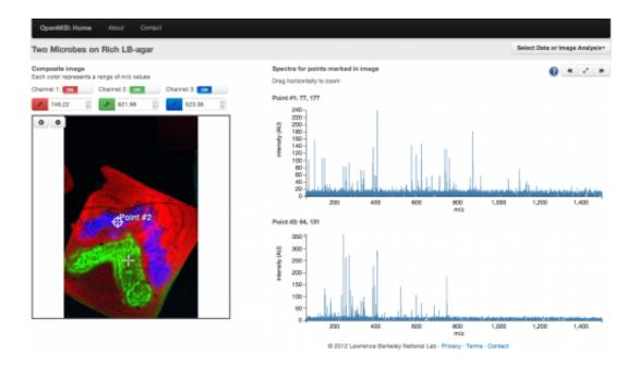
Screen-shot of the OpenMSI online data viewer. A mass spectrometry image is shown on the left. Each pixel in this image is literally packed with information. This information is displayed as a complex spectrum (shown on the right) where each peak indicates the presence of a molecule. As researchers click around the image, the spectrum changes to show the molecules packed withing the selected pixel. Credit: Oliver Ruebel and Ben Bowen (Berkeley Lab)
